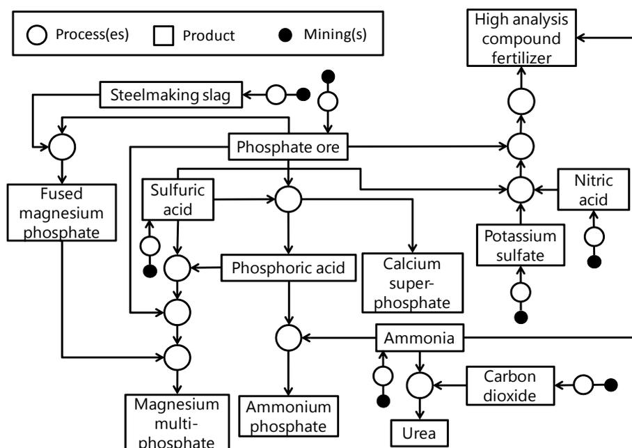
Fig. 1 Schematic diagram of the process flow for phosphate fertilizer production.
